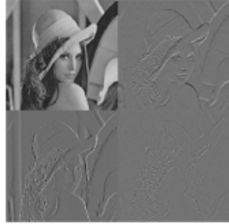
Figure 1. An example of one level discrete wavelet transform. From upper left (clockwise), A_{LL} , A_{LH} , A_{HL} , and A_{HH} .
