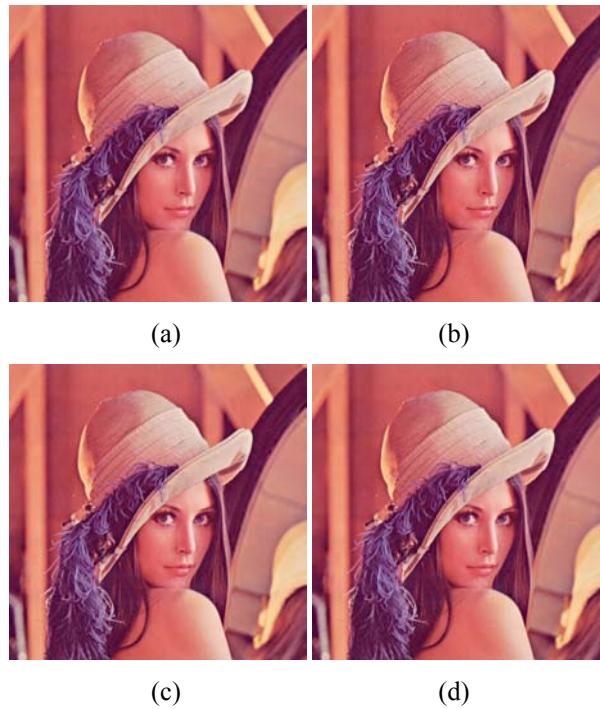
Fig. 7. Lena embedded using recursive, quad-based algorithm (a) original, (b) 28.61 dB embedded with 1,003,843 bits, (c) 33.48 dB embedded with 588,880 bits, (d) 37.15 dB embedded with 309,567 bits.
